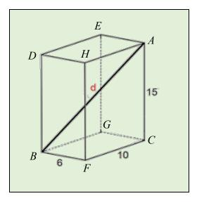
To calculate the diagonal that connects A to B is also the hypotenuse of the right-angled triangle, *ABC*.
