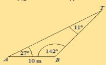
We can now find the length of TB by using the sine rule in  $\Delta TAB$ .
