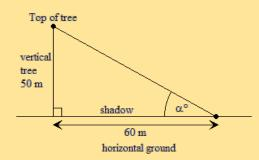
With reference to  $\propto$ , the opposite and adjacent sides of the triangle are 50 m and 60 m respectively. Hence, we may use the tangent ratio,
